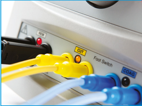
Figure 17 - Connection panel for the cut and coag footswitch control on the Rigel Uni-Therm
