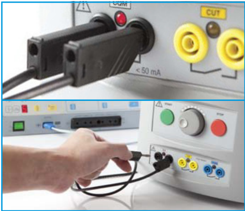
Figure 10 – Connecting Rigel Uni-Therm to the CQM circuit
