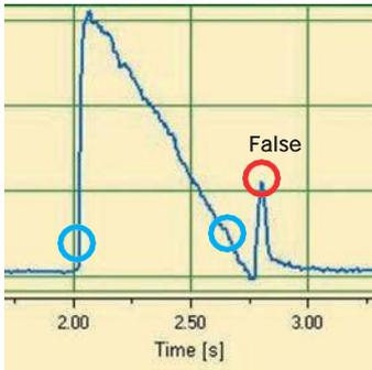
This graph shows the flow curve in the inspiratory channel upstream of the Y-piece. The first two circles indicate the triggers that should be used in this case.
