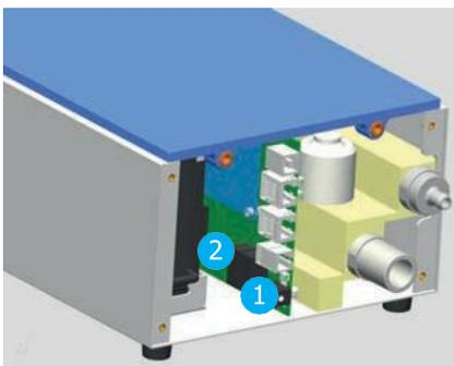
1. 250 VAC, 300 VDC, 1.25 A F, 5×20 (external supply 18 V)
