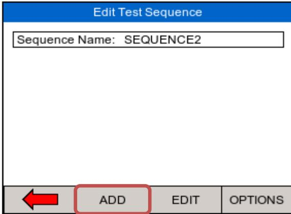
Note: When no individual tests are inserted, the EDIT and OPTIONS buttons are not active
