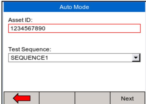
When using the barcode scanner, ensure the barcode scanner is paired with the Rigel Uni-Therm, see Chapter 7. (The Rigel Uni-Therm will only support the Seaward barcode scanner, p/n 339A923). When the barcode is ready to scan, the word "OK" will appear in the asset ID field.
