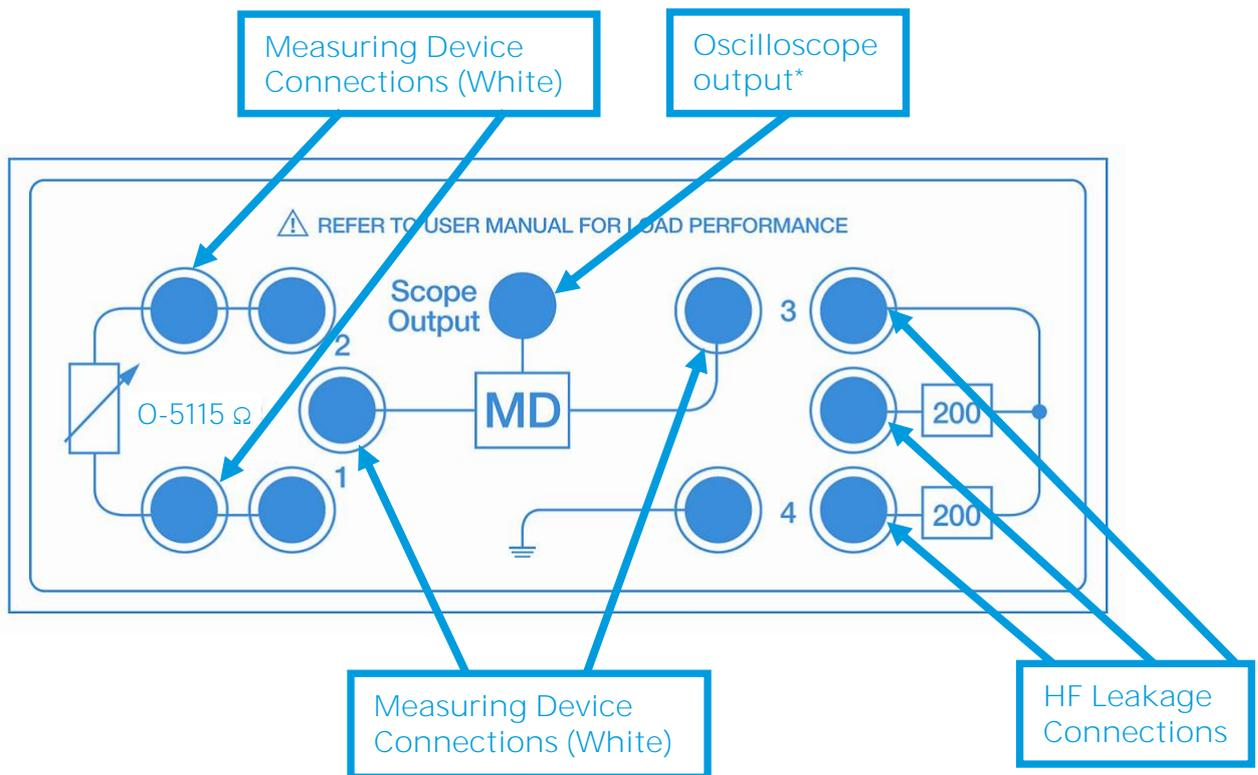
\*Note: The scope output (SMB connector) provides an 10kV isolated waveform monitoring output however the scope output is not calibrated.
