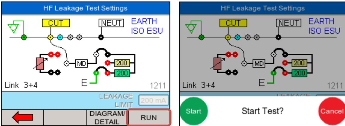
Follow the connection instructions on the main screen and press RUN to confirm and start the HF leakage test. The next step is a custom test to instruct the user to set the output power to maximum (300W) in this example.
