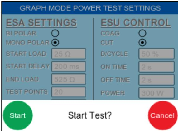
Press the GREEN button to start the test. The Rigel Uni-Therm will now activate the EUT through the foot paddle control on the front panel.
