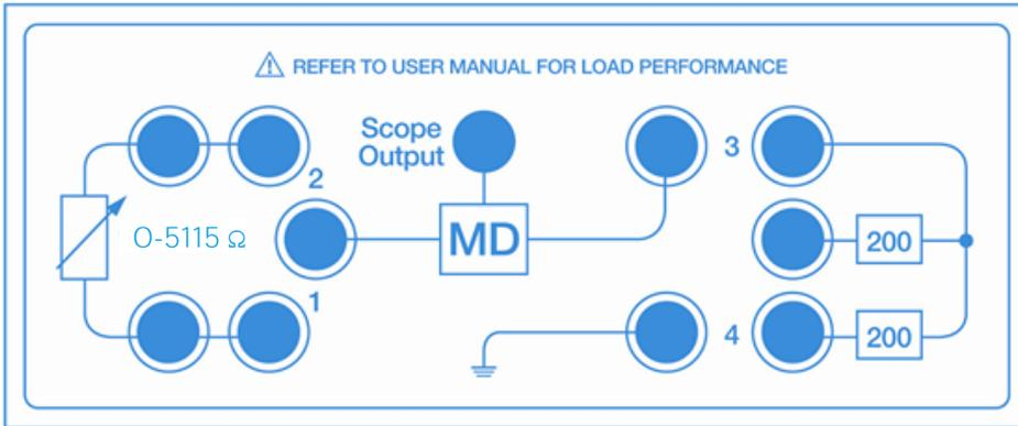
Follow the on-screen instruction diagrams for correct test connection. See appendices A and B for embedded connection diagrams. Connect the ESU active and neutral electrodes to the side panel as indicated, also fit jumper links (positions 1, 2, 3, 4) as required to complete circuits.
