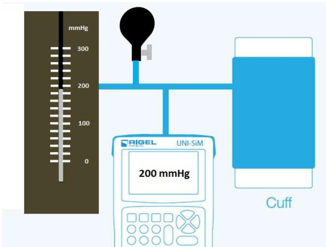
*Figure 1. Sphygmomanometer test setup*
