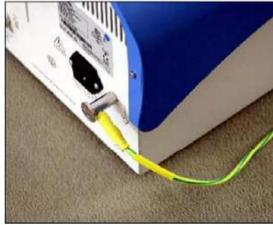
Note: For utilizing the Uni-Therm, connect the patient return of the generator to the left white jack on the side of the Uni-Therm. Connect the right side white jack to the rear ground lug of the generator.
