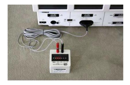
Note: Rather than the need for an external decade box, the Uni-Therm's REM load provides the variable resistance needed.
