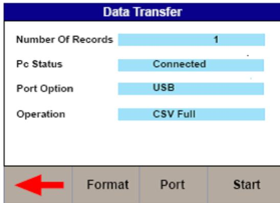
3) Then the correct Operation must be chosen. The operations are divided into Export or Import and also into format or type of file e.g. SSS, CSV Full, CSV Summary, Test Sequence, Results, Ref Graph. The user will need to select the appropriate operation which for downloading results would be Export SSS and then press Start.
