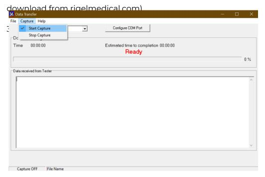
Figure 1. Start capture on DataTransfer.exe
