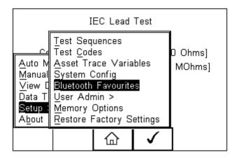
2) Scroll to the device type you are attempting to connect to (barcode, printer or computer) and press F3 for set up
