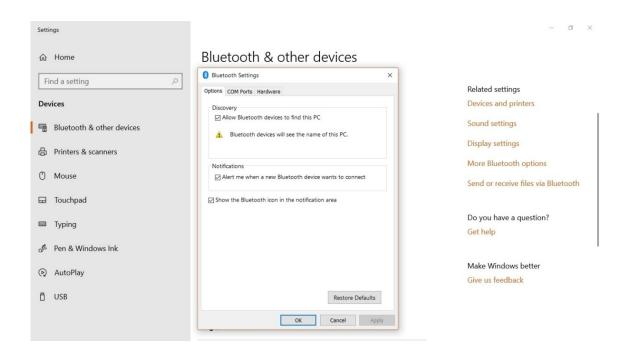
Add the tester and wait for it to confirm that it has been paired successfully. It may be a requirement to have the free Data Transfer program or Rigel Med-eBase open during pairing. Both are downloadable from our website.
