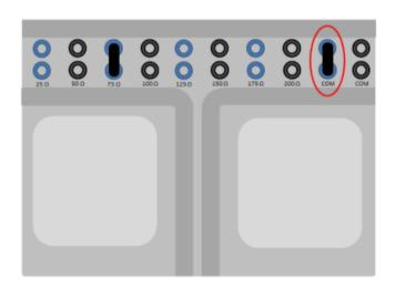
The selected resistance of the variable load box will appear on the UNI-PULSE when the OHM button is pressed;
