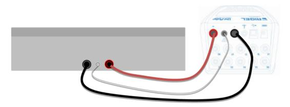
When used in combination with the Rigel UNI-PULSE, the grey wire is the sense cable and will allow the UNI-PULSE to measure the set resistance to help avoid incorrect test setup.
