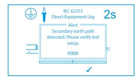
If the secondary earth paths cannot be removed, one should revert to the differential leakage method in IEC 62353, which can measure the total leakage even when a secondary earth path exists. This is because the differential leakage method does not rely on a 1kD body model.
