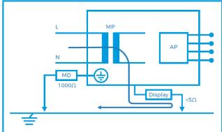
This will result in a zero reading on the safety analyser and could potentially pass a dangerous medical device. In case a secondary earth path exists, the Rigel safety analysers will provide the user with an error message.
