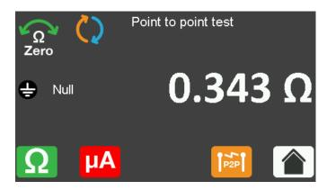
Select  $\Omega$  to perform a point to point ground bond test
