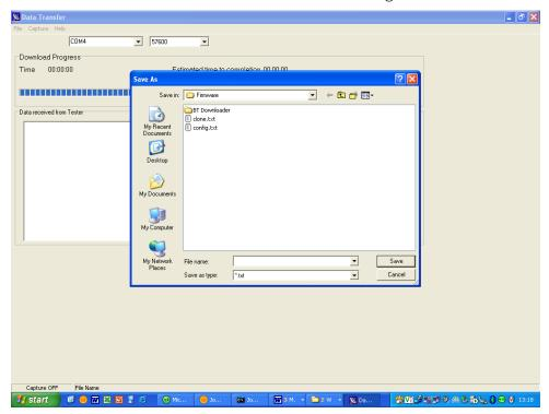
Once the text file has been created, press the Send button (F4) to transfer the Asset Trace variables and User names from the Rigel 288 plus to the PC.
