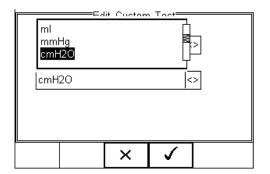
To insert the new Custom Test, press the button (F4) or exit using the button (F3) and return to the previous screen without changes being made.
