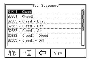
From this menu, the user is able to View a test sequence by pressing the View button (F4). Default test settings cannot be altered at any stage.
