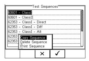
Use the Up & Down Arrow keys to select the required action and press the confirm. Press Escape (F3) to cancel and return to previous screen. (F4) to
