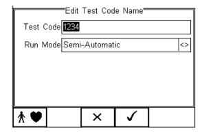
Enter a 4-digit Test Code, in this example 1234, and use up. Down. Left and right keys to select either Semi-Automatic or Automatic. (See 4.5.1)
