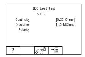
Press (C) button (F3) to set the Pass/Fail limits for Continuity, Insulation and Test Voltage. Use the up, down, left and right keys to highlight and set. The pass/fail limit for the continuity stage can be calculated using the Calc button (F2). Enter the type and length of cable and a new limit will be calculated. This can be overridden by selecting the
