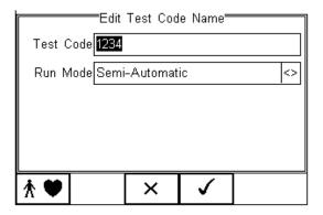
When returning to the Edit Test Code Name screen, confirm and save the Test Code by pressing the button (F4), see below.
