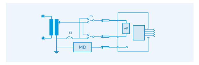
Diagram A - Test Circuit for Earth Leakage
