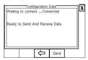
Open the Bluetooth Downloader (Data Transfer.exe) application on your PC and check that the Com Port is correct for the Bluetooth USB adaptor being used with the P.C. The baud rate will default to the correct value of 57600. If an RS232 cable is used, please default to a baud rate of 9600. A higher baud rate may result in incorrect data being transmitted.
