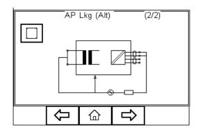
The test is performed using a current limited (3.5mA) mains potential sinusoidal 50Hz signal. (60Hz where this is the mains frequency)
