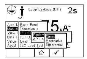
Use the Up, Down, Left and Right keys to navigate through the menu and press the button (F4) to confirm.
