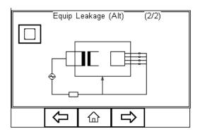
The test is performed using current limited (3.5mA) mains potential sinusoidal 50Hz signal. (60Hz where this is the mains frequency)
