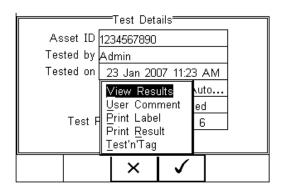
**View Results** will display the results of the test (see section 4.9)
