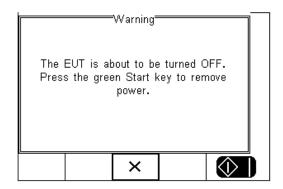
Now the test sequence requires to open the Neutral which will result in a power break. The Semi Automatic mode provides the user with a warning and requires a confirmation prior to interrupting the Neutral. This allows the user to properly power down the Medical Device and prevent possible damage caused by interupting the power supply.
