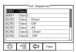
From this menu, the user can create a new Test Sequence by pressing the butto (F1).
