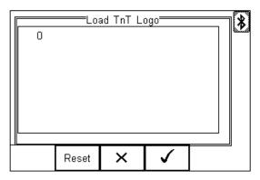
The Rigel 288 plus is now ready to receive data. The amount of data received is shown numerically on the top left of the display (0 in the screen shot above).
