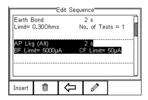
Further electrical safety tests can be inserted or deleted by following the steps described herein.
