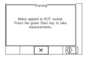
The next step is to reverse the power supply. The Rigel 288 plus will automatically reverse the power and start the test sequence again. In the semi-automatic mode, the user can determine when the measurements start. In full automatic mode, the power reversal is instant and measurements will start directly after mains reversal.
