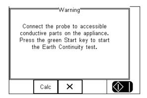
Attention! Ensure the earth bond test lead is connected to the lower (black) 4 mm socket when testing between probe and EUT earth.
