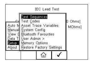
The following overview is provided and shows the list of default and customised test sequences available. Copied Test Sequences will appear in the list with an \*pre-fix.
