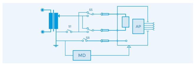
Diagram B - Test Circuit for Enclosure Leakage
