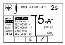
Note: Below is a map showing where the individual tests can be selected in the Manual Mode menu.
