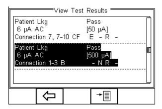
Use the button (F2) to return to the Test Details screen. The button (F4) provides extra option to print results, label or Test 'n tag
