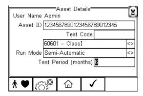
6. Configure the Applied Part module when required by pressing the \*\bigam \bigcup button (F1).
