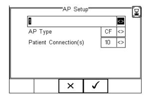
Edit the first line or use the up, down, left and right keys to select from a list of default names. Any new name entered will be added to the default list for future reference.
