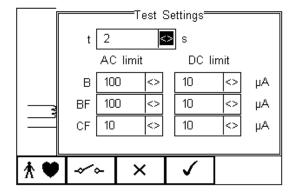
To configure the Applied Part Module press the button (F1) in the Settings menu. For instructions on using this feature, see 4.5 point 6
