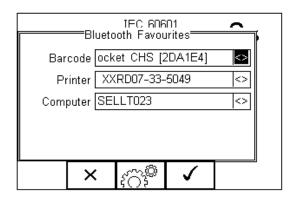
"SELLT023" is now a Bluetooth Favourite, and the Rigel 288 plus will automatically establish a connection with "SELLT023" when using functions that communicate with a computer e.g., downloading records to a PC database software package.
