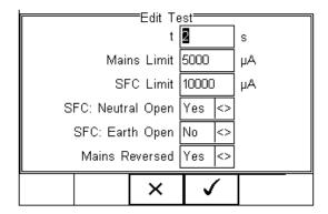
Highlight the required field using the up and down keys. To change the content either use the left and right keys or use the keypad to enter the correct data. To Delete the field content, press the button as shown below.
