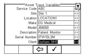
8. Use the Up & Down Keys to navigate the menu and the Left & Right Keys to open the drop down boxes [<>]. Select the required input and confirm with the button (F4). Each variable entered during the automatic test will automatically be added to the list for future use. Trace Variables that are de-activated (set to NO in the Setup menu, section 0) will not appear during the automatic tests.
