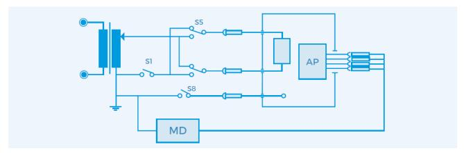
Diagram C - Test Circuit for Patient Leakage Current
