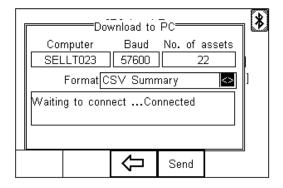
Initially, the Bluetooth status icon will display the egg timer for a few seconds, as shown on the left, while the connection is established. When the connection is established and ready to communicate the Bluetooth status icon will change to show the Bluetooth icon as shown on the right.
