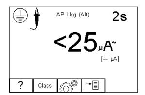
Press (C) button (F3) to set the Test Duration and Pass/Fail limit. Use the up, down, left and right keys to highlight and set. Press button (F4) when complete. Pressing
