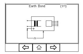
If an earth bond lead other than that supplied with the Rigel 288 plus is to be used then any resistance associated with this lead can be zeroed out by connecting the supplied earth bond lead to the EUT earth socket on the Rigel 288 plus and pressing the zero button (F2). If the zero function has been activated, then the zero icon overwrites the single probe icon in the top left of the display. By preventing the zero button (F2) again this function is cancelled.
