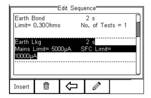
Once the Insert button (F1) has been pressed, a drop-down box will appear with all available safety tests and inspection available. Activate the drop-down box using the left key and select the Custom Test option.
