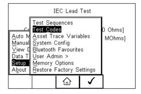
Press the button (F4) to select Test Codes. Press the button (F3) to return to the Home screen.
