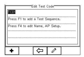
Press the button (F4) to allocate a unique 4-digit code and or to configure the Applied Part setup and test mode to Semi or Full Automatic.
