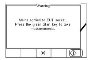
This example uses the Semi Automatic Mode and the user has the opportunity to determine the moment at which the leakage measurements start. In fully automatic mode, the Rigel 288 plus will start the measurements immediately after the EUT has been switched on.
