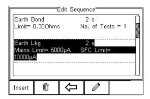
Once the Insert button (F1) has been pressed, a drop-down box will appear with all available safety and inspection tests. Activate the drop-down box using the left key and or scroll through the available tests using the up and down keys.
