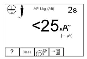
Press (C) button (F3) to set the Test Duration, Equipment Class, Applied Part module and RMS Pass/Fail limit for BF and CF Applied Parts. Use the up, down. left and right keys to highlight and set. Press (F4) when complete. Pressing the will exit Settings mode without saving changes.
