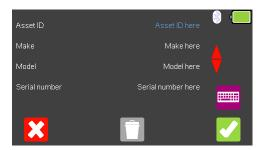
To confirm the asset details, select  $\checkmark$  (F5). Once information is entered, data on an individual line can be deleted using the  $\checkmark$  (F3) key or to exit without creating an asset select  $\checkmark$  (F1).
