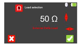
To exit without changing select (F1). Use the (F1) key to select either the Internal Defib Load (fixed at  $50\Omega$ ) or External Defib Load (variable between 25 and  $200\Omega$ ), use the
