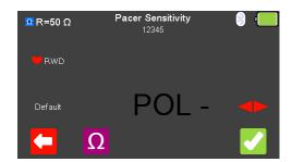
The Polarity of the Pacer Sensitivity can be selected using the arrow key.
