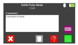
At the end of a test select (F5) to save, additional comments can be added using the keyboard, entered data can be deleted using the (F3) key.
