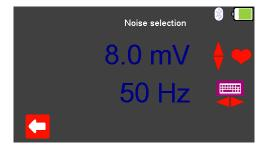
Select (F3) to change the Noise selection to a fixed value between OmV to 10.0mV and a frequency of either 50Hz or 60Hz (using the arrow keys), changes are made using the arrow keys, selecting (F1) confirms this selection.
