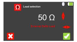
To exit without changing select (F1). Use the (F1) key to select either the Internal Defib Load (fixed at  $50\Omega$ ) or External Defib Load (variable between 25 and  $200\Omega$ ), use the
