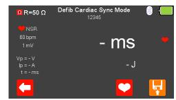
From the Defib Pulse Mode menu select (F4) for Defib Cardiac Synch Mode. The UniPulse 400 is now ready to measure the cardiac synchronisation time.
