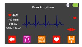
The Heart rate, Amplitude, and Noise settings are displayed on the left-hand side of the display.
