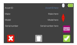
To confirm the asset details, select  $\checkmark$  (F5). Once information is entered, data on an individual line can be deleted using the  $\Box$  (F3) key or to exit without creating an asset select  $\checkmark$  (F1).
