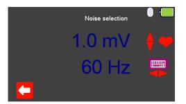
Select (F3) to change the Noise selection to a fixed value between OmV to 10.0mV and a frequency of either 50Hz or 60Hz (using the arrow keys), changes are made using the arrow keys, selecting (F1) confirms this selection.
