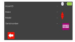
The Asset ID, Make, Model and Serial Number of the appliance under test can be added, to exit without saving select (F1).
