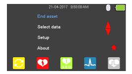
Selecting (F5) returns the instrument to the Main Menu, however, the Start asset option is now displayed as End asset. Note; if End asset is selected the display reverts back to Start asset and the asset details previously entered can no longer be used.
