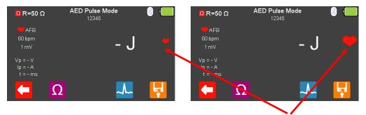
The simulation (output from the UniPulse 400) is active when the red heart symbol is pulsing.
