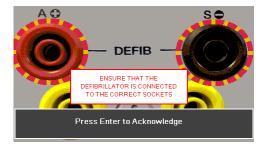
Note<sup>1</sup>: to enter the Defibrillator Pulse or AED mode you have to accept the connections warning, using the  $\downarrow$  (return) key, – the red and black 4mm defibrillator terminals are highlighted with a flashing red / yellow image.
