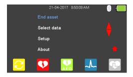
Selecting (F5) returns the instrument to the Main Menu, however, the Start asset option is now displayed as End asset. Note; if End asset is selected the display reverts back to Start asset and the asset details previously entered can no longer be used.
