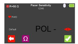
The Polarity of the Pacer Sensitivity can be selected using the arrow key.
