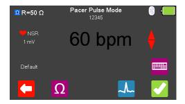
From the Pacer Pulse Mode select (F4) to alter the simulation waveform selection. Use the arrow keys to move between the available simulation waveforms.
