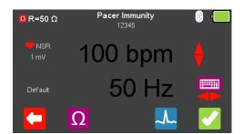
From the Pacer Immunity Menu select (F4) to alter the simulation waveform selection. Use the arrow keys to move between the available simulation waveforms.
