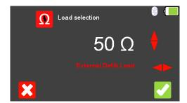
To exit without changing select (F1). Use the  $\Rightarrow$  arrow keys to select either the Internal Defib Load (fixed at  $50\Omega$ ) or External Defib Load (variable between 25 and  $200\Omega$ ,
