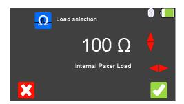
To exit without changing select (F1). Use the (F1) key to select the Internal Pacer Load (variable between 50 and (F1)), use the (F1) arrow keys to select the load resistance. To confirm the load select (F5) or exit without changing the resistance by selecting (F1).
