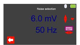
Select (F3) to change the Noise selection to a fixed value between OmV to 10.0mV and a frequency of either 50Hz or 60Hz (using the arrow keys),
