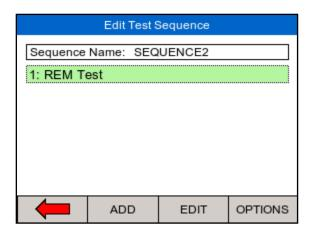
Repeat the above steps until the required test sequence is completed. Note that additional tests can be inserted in the test sequence by highlighting the position in the sequence and press the ADD (F2) button. The test will be inserted AFTER the highlighted position.
