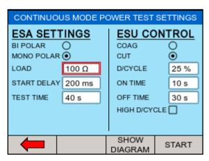
Use the rotary encoder to navigate the screen. The selected field is marked with a red border, presses the rotary encoder to activate the field to allow changes. Confirm and deactivate the field by pressing the encoder once again.
