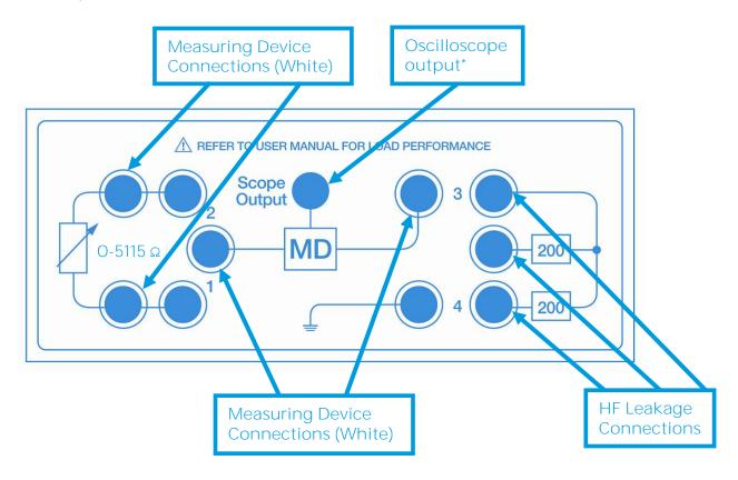
\*Note: The scope output (SMB connector) provides an 10kV isolated waveform monitoring output however the scope output is not calibrated.
