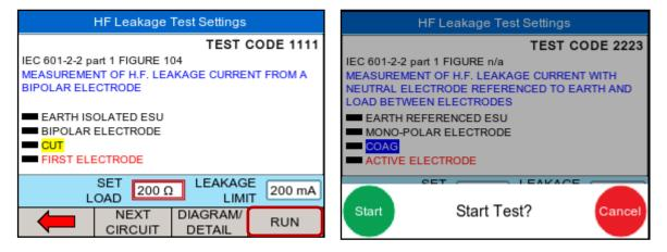
The Rigel Uni-Therm could display the following details after the test;
