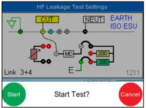
Follow the connection instructions on the main screen and press RUN to confirm and start the HF leakage test. The next step is a custom test to instruct the user to set the output power to maximum (300W) in this example.
