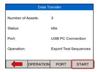
Press start to connect the Uni-Therm as an external drive to the PC.
