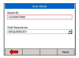
When using the barcode scanner, ensure the barcode scanner is paired with the Rigel Uni-Therm, see Chapter 7. (The Rigel Uni-Therm will only support the Seaward barcode scanner, p/n 339A923). When the barcode is ready to scan, the word "OK" will appear in the asset ID field.
