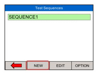
Select NEW (F2) to open a new test sequence and enter a name, use the rotary encoder or USB keyboard to enter data; Select KEYBOARD to change the format from QWERTY to ABCD style;
