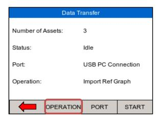
Change between USB Memory Stick or Cable, using the PORT (F3) key.
