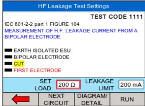
The rotary encoder can be used to scroll the different test setups, or to SET LOAD and LEAKAGE LIMIT values. The selected field is highlighted in red. Press the rotary encoder to activate the field (field turn blue) and use the rotary encoder to change the settings. Press the rotary encoder again to confirm
