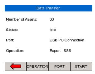
Change between USB Memory Stick or Cable, using the PORT (F3) key.
