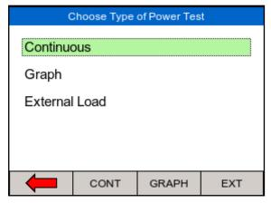
Select Power test from the home screen; then select F2 (CONT) F3 (GRAPH) or F4 (EXT) modes using the fast keys; to select either the Continuous, Graph or External Load test. Use the rotary encoder or the dedicated function keys to navigate.
