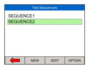
Edit Sequence Name, Copy or Delete the test sequence from the Test Sequences menu, select OPTION:
