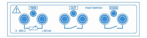
For automatic control during HF leakage and Power tests, connect the ESU footswitch COAG and CUT contacts to the blue and yellow terminals.
