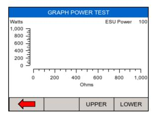
Select the UPPER and LOWER limit graphs by pressing UPPER and LOWER respectively and select the corresponding graphs;
