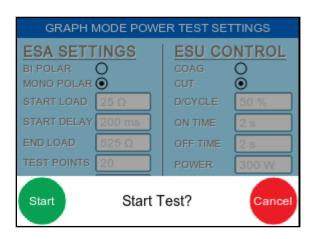
Press the GREEN button to start the test. The Rigel Uni-Therm will now activate the EUT through the foot paddle control on the front panel.
