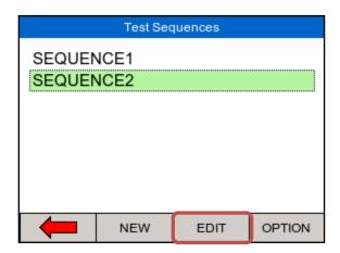
Press the EDIT (F3) button to open the test sequence for editing;
