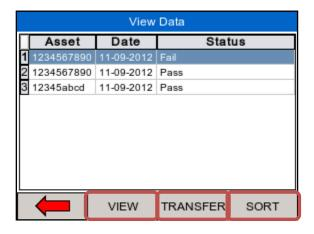
Data can be sorted using the SORT (F4) key which will sort on asset number and date either ascending or descending.
