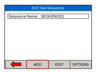
Note: When no individual tests are inserted, the EDIT and OPTIONS buttons are not active Start adding individual tests to the test sequence by pressing the ADD (F2) button;
