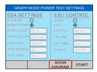
The Rigel Uni-Therm will display the settings. Press SHOW DIAGRAM (F3) to show the connection diagram;
