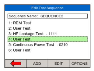
The individual tests can now be edited / configured to the specific requirements. Once an individual test has been configured, they can be copied and pasted repeatedly by selecting the OPTIONS button.
