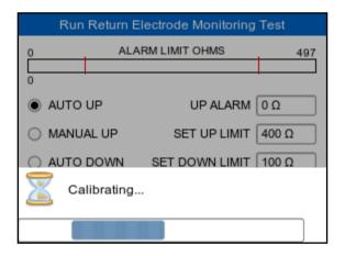
Once the calibration has completed, the CQM / REM test screen will appear;
