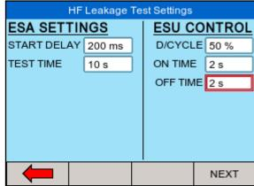
Press NEXT to confirm and start selecting the appropriate leakage tests.
