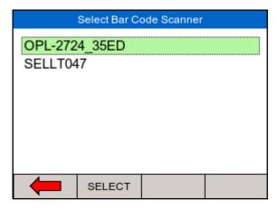
To pair the appropriate device to the corresponding function, select and open the drop-down box using the rotary encoder and press SELECT for each correct device;
