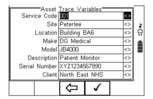
6. Use the Up & Down Keys to navigate the menu and the Left & Right Keys to open the drop down boxes [<>]. Select the required input and confirm with the
