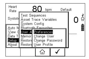
Navigate through this menu using the Up & Down Keys and select by pressing the button (F4) or the right arrow key.
