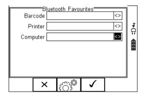
Use the up/down arrow keys to highlight the device type (in this case Computer) then press (F3).
