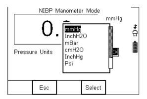
The manometer will automatically convert the pressure to the desired pressure unit.
