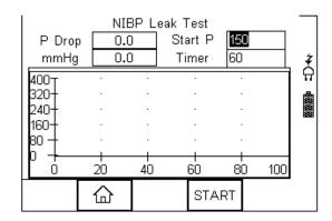
The BP-SIM will inflate the system to around the set-point. Once the system is stabilised at the set pressure, the timer will count up for the set duration. This is highlighted below:
