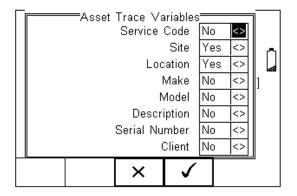
The default settings on the Rigel BP-SIM include the Site and Location variables. Both are activated. The drop down box is set to [Yes].
