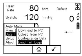
The Rigel BP-SIM will now attempt to connect to the PC, setup in Bluetooth Favourites. When a connection has been established the display will be as shown below.
