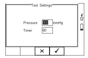
Highlight the required field using the up and down keys. To change the content use the keypad to enter the correct data. To Delete the field content, press the button as shown below.
