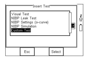
Confirm using the button (F4). The following menu will define the nature of the test (eg test Instruction prior to leak test)
