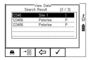
Use the up and down arrow keys to scroll through the database. When the desired record is highlighted, press the button (F4) to enter the record and view the data.
