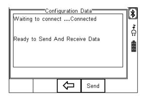
Press the SEND (F4) button to send data to the PC.
