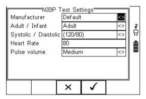
Navigate using the Up & Down Keys and change each setting by using the left key.
