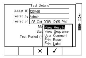
Use the up and down keys to select the view results option. Press the (F4) to display the view text results screen (see below).
