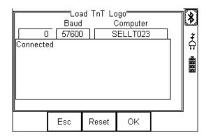
The Rigel BP-SIM is now ready to receive data. The amount of data received is shown numerically on the top left of the display (0 in the screen shot above).
