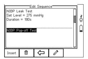
Once the Insert button (F1) has been pressed, a drop down box will appear with all available tests and inspection available. Activate the drop down box using the left key and select the Custom Test option.
