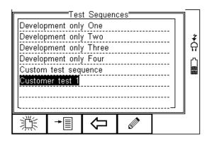
Once the Test Sequence has been opened, individual tests can be inserted by highlighting the place where a new test needs inserting using the up and down keys.
