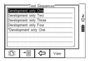
From this menu, the user is able to create a new Test Sequence by pressing the button (F1).
