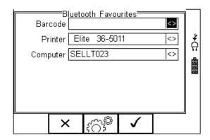
"SELLT023" and "Elite 36-5011" are now a Bluetooth Favourite and the Rigel BP-SIM will automatically establish a connection with "SELLT023" when using functions that communicate with a computer e.g. downloading records to a PC database software package or connect to "Elite 36-5011" when requiring a print-out.
