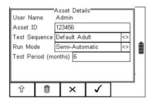
5. Returning to the Asset Details screen, the for button (F2) provides the user with the option to modify or create a new Test Sequence from this menu. This feature is identical to that of the Test Sequence feature in the Setup - Test Sequence menu. (See 3.1 for more information)
