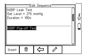
Once the Insert button (F1) has been pressed, a drop down box will appear with all available tests. Activate the drop down box using the left key and or scroll through the available tests using the up and down keys.
