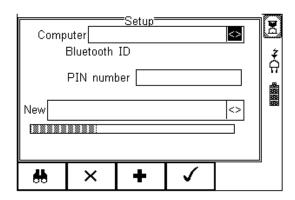
Use the arrow keys to highlight the field labelled "New" and press the left or right keys to open the list of devices which have been found during the search.
