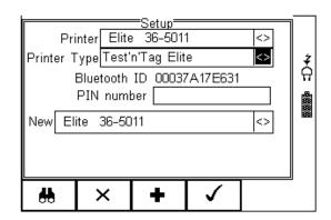
Ensure when selecting the printer, that the Printer type is selected corresponding with the print media:
