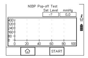
To initiate the test, press START (F4). The BP-SIM will inflate the system until the protection valve is activated;
