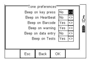
Navigate using the Up & Down Keys and change between Yes / No using the left key.
