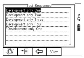
From this menu, the user is able to View a test sequence by pressing the View button (F4). Default test settings cannot be altered at any stage.
