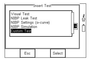
Once the desired test has been highlighted, confirm using the OK button (F4) and finally confirm to insert into the test Sequence. Pressing the button (F3) will return to the previous screen without changes being made.
