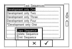
Use the Up & Down Arrow keys to select the required action and press the (F4) to confirm. Press Escape (F3) to cancel and return to previous screen.
