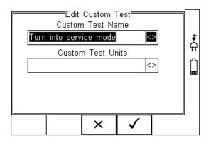
To insert the new Custom Test, press the button (F4) or exit using the button (F3) and return to the previous screen without changes being made.
