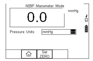
Ensure the manometer is set to zero by pressing the SET ZERO (F3) button) whilst the pressure connection at the BP-SIM panel is open.
