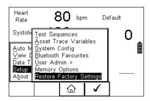
All the settings provided within the Setup menu will default to Factory Settings including; All Asset Trace Variables, Test Sequences, User Admin, Test Codes and System Config.
