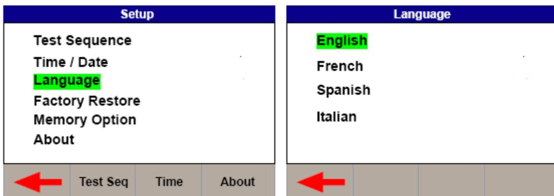
Use the rotary encoder to navigate, push to select the language. Press the back button (F1) to confirm or return to previous menu.
