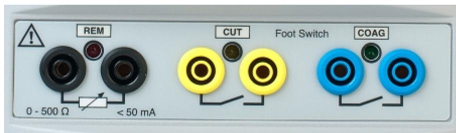
For automatic control during HF leakage and Power tests, connect the ESU footswitch COAG and CUT contacts to the blue and yellow terminals.
