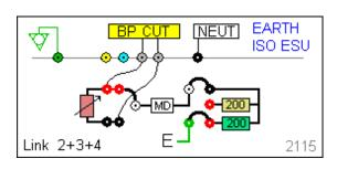
**TEST CODE 2213** IEC 601-2-2 part 1 FIGURE N/A MEASUREMENT OF H.F. LEAKAGE CURRENT WITH **NEUTRAL ELECTRODE** REFERENCED TO EARTH **AND** LOAD **BETWEEN ELECTRODES EARTH** REFERENCED ESU MONO-POLAR ELECTRODE CUT MODE **NEUTRAL ELECTRODE**
