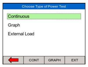
Select Power test from the home screen; then select F2 (CONT) F3 (GRAPH) or F4 (EXT) modes using the fast keys; to select either the Continuous, Graph or External Load test. Use the rotary encoder or the dedicated function keys to navigate.
