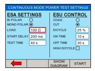
Use the rotary encoder to navigate the screen. The selected field is marked with a red border, presses the rotary encoder to activate the field to allow changes. Confirm and de-activate the field by pressing the encoder once again.
