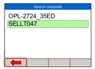
The devices found in range will be listed. Wait until the search has been completed which can take up to 15 seconds. Once the search is completed, press the back arrow key;
