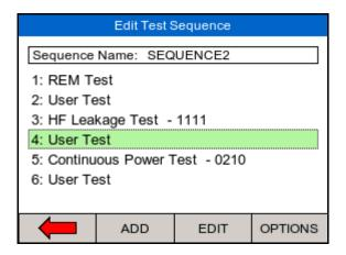
The individual tests can now be edited / configured to the specific requirements. Once an individual test has been configured, they can be copied and pasted repeatedly by selecting the OPTIONS button.
