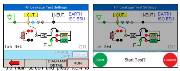
confirm and start the HF leakage test. The next step is a custom test to instruct the user to set the output power to maximum (300W) in this example.
