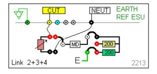
**TEST CODE 2223** IEC 601-2-2 part 1 FIGURE N/A MEASUREMENT OF H.F. LEAKAGE CURRENT WITH **NEUTRAL ELECTRODE REFERENCED** TO EARTH **BETWEEN** AND LOAD **ELECTRODES EARTH** REFERENCED ESU MONO-POLAR ELECTRODE COAG MODE **NEUTRAL ELECTRODE**
