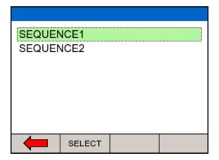
Next, select the Test Sequence box (push to select) and select the required test sequence. (To add new test sequences, see <a href="Chapter 8.1">Chapter 8.1</a>).
