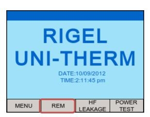
During the initial CQM / REM test selection, the Rigel Uni-Therm will auto-calibrate the CQM / REM potentiometer;
