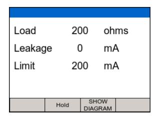
Press the HOLD key to freeze the reading on the screen. The test can be aborted by pressing the red STOP button on the front of the Uni-Therm.
