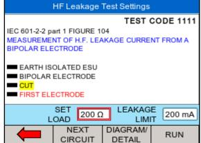
or the IEC 60601-2-2 reference details (SHOW DETAIL). The rotary encoder can be used to scroll the different test setups, or to SET LOAD and LEAKAGE LIMIT values. The selected field is highlighted in red. Press the rotary encoder to activate the field (field turn blue) and use the rotary encoder to change the settings. Press the rotary encoder again to confirm
