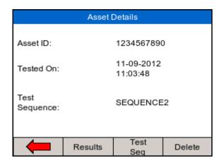
Test results can be viewed by pressing the RESULTS (F2) button, test settings can be viewed by pressing TEST SEQ (F3) button and deleted by pressing the DELETE (F4) button.
