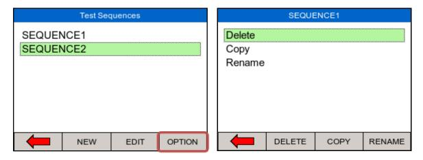
To delete a test sequence, press DELETE To copy a test sequence, press COPY To rename a test sequence, RENAME
