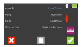
To confirm the asset details select (F5). Once information is entered, data on an individual line can be deleted using the (F3) key or to exit without creating an asset select (F1).
