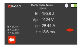
Using the arrow keys allows the various test result screens to be viewed on the UniPulse 400. The format of these depends on the original test performed.
