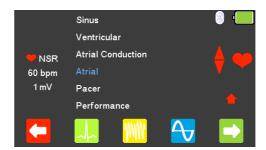
From the Main Menu select (F4) for ECG simulation and highlight Atrial using
