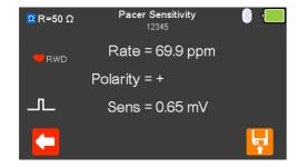
With the EUT pacing, the rate, polarity and sensitivity are displayed.
