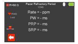
If no pacer signal is received from the EUT then a red cross appears in the pulse waveform.
