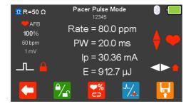
With the EUT pacing, the rate, pulse width, peak current and energy are displayed.
