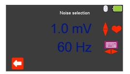
Select (F3) to change the **Noise selection** to a fixed value between 0mV to 10.0mV and a frequency of either 50Hz or 60Hz (using the arrow keys),
