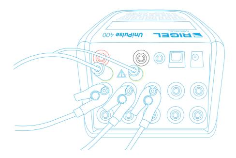
Connect the Pacer leads to the yellow 4mm PACER terminals on the rear of the UniPulse 400.
