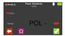
From the **Pacer Menu** use the arrow keys to highlight **Sensitivity** and confirm using the key or select F4).
