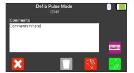
At the end of a test select (F5) to save, additional comments can be added using the keyboard, entered data can be deleted using the (F3) key.
