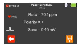
With the EUT pacing, the rate, polarity and sensitivity are displayed.
