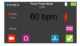
From the **Pacer Menu** use the arrow keys to highlight **Pacer Pulse Mode** and confirm using the  $\downarrow$  (return) key or select (F2).
