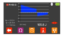
The measured energy will be displayed on the UniPulse 400 screen as well as the peak voltage, peak current and pulse duration.
