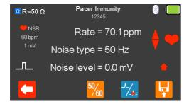
With the EUT pacing, the rate, noise type and noise level are displayed.
