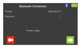
Select (F5) to connect to the printer, once connected, **Printer ready** and the Bluetooth icon are displayed, and selecting (F5) prints the result.
