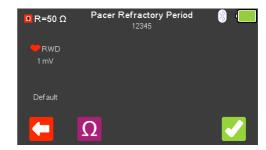
From the **Pacer Menu** use the arrow keys to highlight **Refractory Period** and confirm using the  $\downarrow$  (return) key or select (F3).
