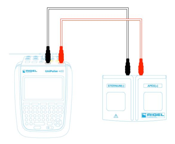
Connect the Paddle Adaptor Box using the red and black 4mm leads to the DEFIB terminals on the rear of the UniPulse 400.
