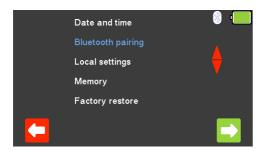
From the **Setup Menu**, use the arrow keys to highlight **Bluetooth pairing** and select using the  $\downarrow$  (return) key or (F5). Ensure the Test 'n' Tag Elite 2 Printer / Bluetooth Scanner is switched on.
