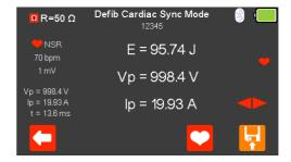
Press (F5) to save the test result or (F1) to exit.
