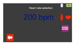
Select (F4) to change the **Heart rate selection** to values between 20 and 300 BPM, selecting (F1) confirms this selection. Note; values can be typed in using the keyboard and either saved using (F5) or cancelled with (F1).
