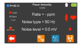
If no pacer signal is received from the EUT then a red cross appears in the pulse waveform.
