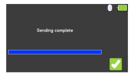
Select (F5) to send the data from the UniPulse 400 connected to a PC via the USB lead.
