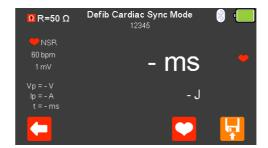
From the **Defib Pulse Mode** menu select (F4) for **Defib Cardiac Synch Mode**. The UniPulse 400 is now ready to measure the cardiac synchronisation time.
