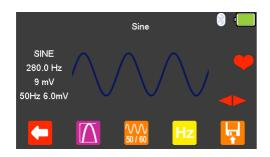
The new **Frequency**, **Amplitude** and **Noise** settings are displayed on the left hand side of the display.
