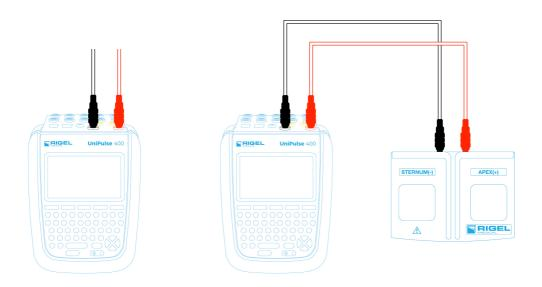
The defibrillator or AED under test can be connected direct to the UniPulse 400 using 4mm connectors, or the Paddle Adaptor Box can be used as shown above.
