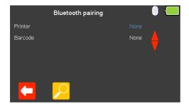
Use (F1) to exit the **Bluetooth pairing** setup screen without saving. The search function (F2) can be used to search for Bluetooth devices.
