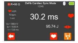
The cardiac synchronisation time will be displayed on the UniPulse 400 screen as well as the measured energy, peak voltage, peak current and pulse duration.
