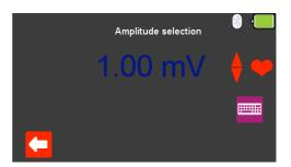
Use the arrow keys to move between the available simulation waveforms. If applicable, select (F2) to change the **Amplitude selection** to a fixed value
