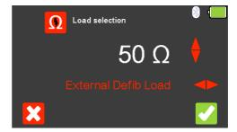
$200\Omega$ , use the  $\bigcirc$  arrow keys to select the external Defib load resistance). To confirm the load select  $\bigcirc$  (F5) or to exit without changing the resistance select  $\bigcirc$  (F1).
