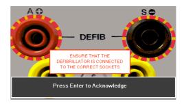
Note 1; to enter the Defibrillator Pulse or AED mode you have to accept the connections warning, using the  $\d$  (return) key, – the red and black 4mm defibrillator terminals are highlighted with a flashing red / yellow image.
