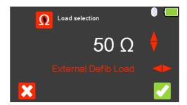
To exit without changing select (F1). Use the (F1) key to select either the **Internal Defib Load** (fixed at  $50\Omega$ ) or **External Defib Load** (variable between 25 and
