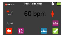
From the **Pacer Pulse Mode** select (F4) to alter the simulation waveform selection. Use the arrow keys to move between the available simulation waveforms.
