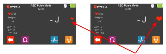
The simulation (output from the UniPulse 400) is active when the red heart symbol is pulsing.
