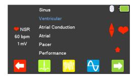
From the **Main Menu** select (F4) for ECG simulation and either select (F3), or highlight **Ventricular** using the arrow keys and confirm using the (return) key or select (F5).
