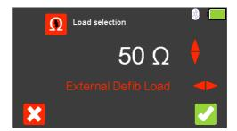
To exit without changing select (F1). Use the (F1) key to select either the **Internal Defib Load** (fixed at  $50\Omega$ ) or **External Defib Load** (variable between 25 and
