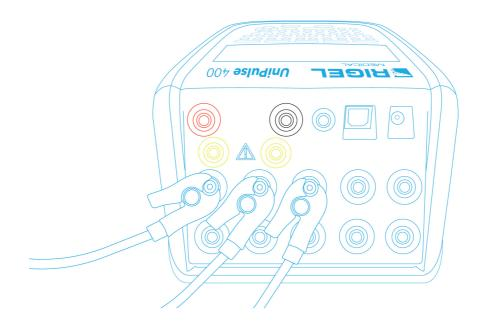
Use the supplied ECG snap connectors to connect ECG leads to the 4mm ECG terminals on the rear of the UniPulse 400. The ECG connectors are colour coded as per international standards.
