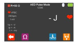
Select (F4) to change the output waveform of the UniPulse 400.
