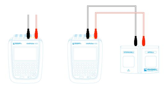
The defibrillator or AED under test can be connected directly to the UniPulse 400 using 4mm connectors, or the Paddle Adaptor Box can be used as shown above.
