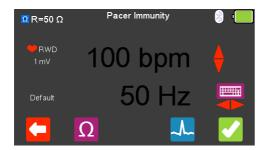
From the **Pacer Immunity** Menu select (F4) to alter the simulation waveform selection. Use the arrow keys to move between the available simulation waveforms.
