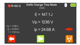
The measured energy will be displayed on the UniPulse 400 screen as well as the peak voltage, peak current and pulse duration. Select the key to view the waveform graph and a measurement summary. Select (F5) to save the test result or (F1) to exit.
