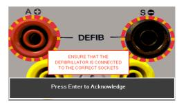
To enter the **Defibrillator Pulse mode** you have to accept the connections warning, using the  $\[ \downarrow \]$  (return) key, – the red and black 4mm defibrillator terminals are highlighted with a flashing red / yellow image.
