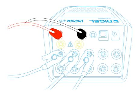
Connect the Pacer leads to the red and black 4mm DEFIB terminals on the rear of the UniPulse 400.
