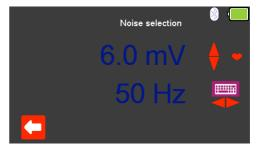
Select (F3) to change the **Noise selection** to a fixed value between 0mV to 10.0mV and a frequency of either 50Hz or 60Hz (using the arrow keys), changes are made using the arrow keys, selecting (F1) confirms this
