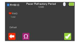
From the **Pacer Menu** use the arrow keys to highlight **Refractory Period** and confirm using the  $\downarrow$  (return) key or select (F3).
