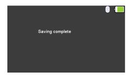
Once all of the information has been entered either select (F5) to save the test as a pass or select (F4) to save the test as a fail. A message will be displayed to confirm **Saving complete** in either case.
