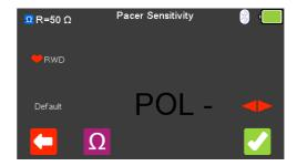
From the **Pacer Menu** use the arrow keys to highlight **Sensitivity** and confirm using the  $\downarrow$  key or select [F4].
