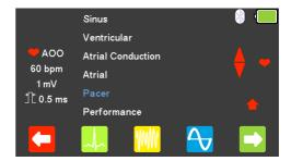
From the **Main Menu** select (F4) for ECG simulation and highlight **Pacer** using the arrow keys and confirm using the (return) key or select (F5).
