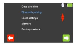
From the **Setup Menu**, use the arrow keys to highlight **Bluetooth pairing** and select using the  $\d$  (return) key or (F5).
