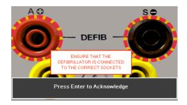
Note 1; to enter the Defibrillator Pulse or AED mode you have to accept the connections warning, using the  $\downarrow$  (return) key, – the red and black 4mm defibrillator terminals are highlighted with a flashing red / yellow image.
