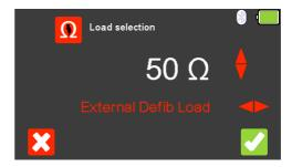
To exit without changing select (F1). Use the key to select either the **Internal Defib Load** (fixed at  $50\Omega$ ) or **External Defib Load** (variable between 25 and
