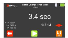
To accurately measure charge time the defibrillator charge must be initiated at exactly the same time as (F3) is selected to begin the timer.
