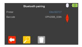
Highlight the Bluetooth printer or scanner to be deleted using the 4 arrow keys. Delete using the (F3) key and then confirm using (F5).
