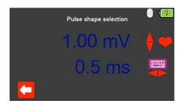
If applicable, select (F2) to change the **Pulse shape selection** to a fixed amplitude between 0.5mV to 5.0mV, changes are made using the arrow keys. Selecting (F1) confirms this selection.
