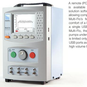
A remote (PC) control interface is available via Rigel's test solution software, Med-eBase, allowing complete control of the Multi-Flo's features from the comfort of a PC. Requiring just a single USB connection per Multi-Flo, the total number of pumps under simultaneous test is limited only by the number of USB ports available. Perfect for high volume test environments.
