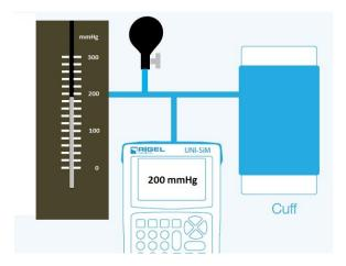
In the picture above, a manual inflator bulb is used to create a positive pressure in the NIBP line which includes the NIBP cuff, the Rigel BP-SIM or UNI-SIM and the Sphygmomanometer.
