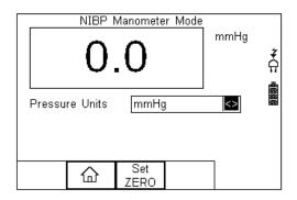
Then apply the required pressure with the bulb and the Rigel BP-SIM or UNI-SIM will show the pressure on the screen which can be compared with the reading on the sphygmomanometer.
