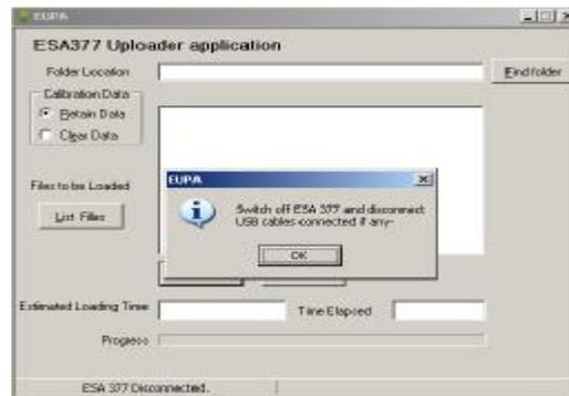
3.3 Connect the USB cable between the PC and the ESA377. The application will automatically find the COM port to which ESA 377 is connected and will display the same in the status bar.
