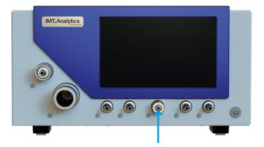
Measuring range: -1-10 bar Accuracy:  $\pm 1$  % of reading or  $\pm 7$  mbar
