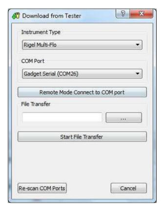
2) Once the software is opened in remote control. Set up the occlusion test as a Manual Occlusion by select the correct channel and then Add Occlusion test. Select Start test and assign the test to an Asset ID.
