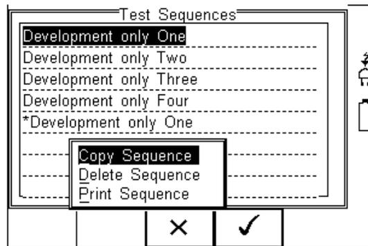
Use the Up & Down Arrow keys to select the required action and press the
