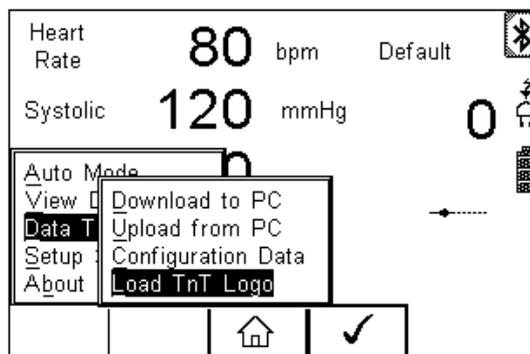
The Rigel BP-SIM will now attempt to connect to the PC, setup in Bluetooth Favourites. When a connection has been established the display will be as shown below.
