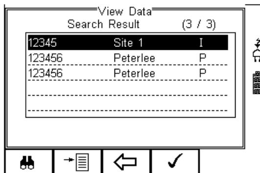
Use the up and down arrow keys to scroll through the database. When the desired record is highlighted, press the
