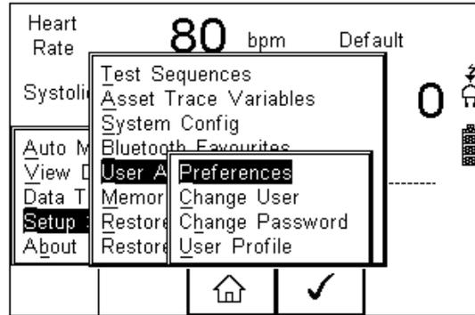
Navigate through this menu using the Up & Down Keys and select by pressing the
