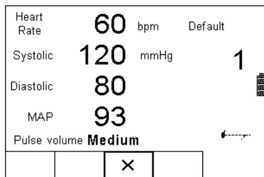
Pressing the **X** (STOP) button (F3) during any test will bring up the failure menu (see 4.1.1)
