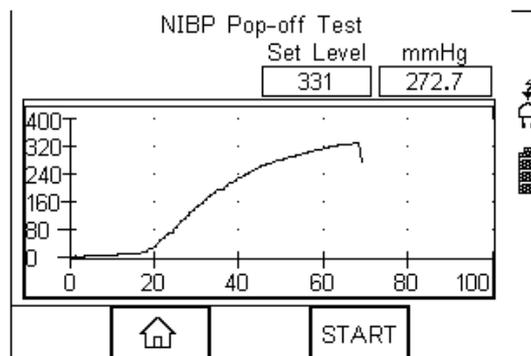
At the end of the test, the BP-SIM will show the set-point of the protection valve (ie 331 mmHg)
