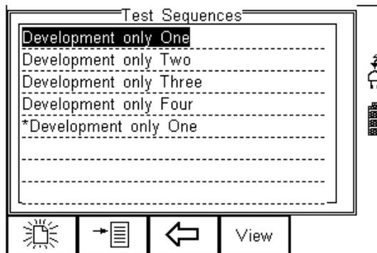
From this menu, the user is able to create a new Test Sequence by pressing the
