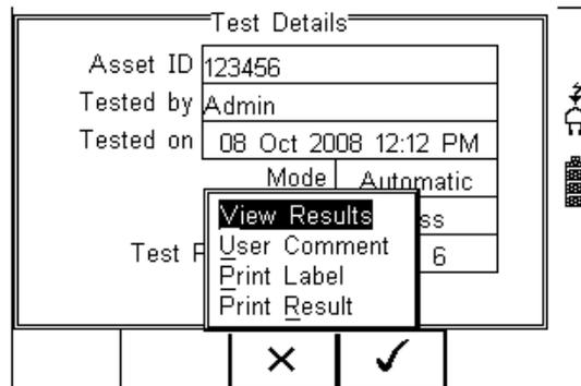
**View Results** will display the results of the test (see section 4.4)
