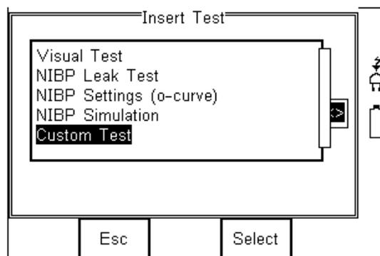
Once the desired test has been highlighted, confirm using the OK button (F4) and finally confirm to insert into the test Sequence. Pressing the **X** button (F3) will return to the previous screen without changes being made.
