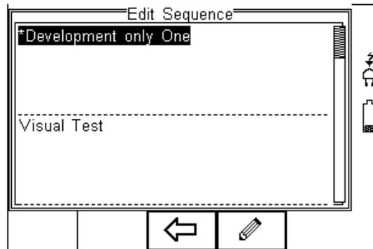
To change the Name and or Class of the Test Sequence, press the
