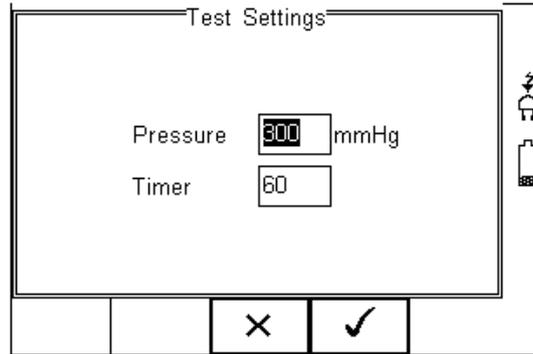
Highlight the required field using the up and down keys. To change the content use the keypad to enter the correct data. To Delete the field content, press the
