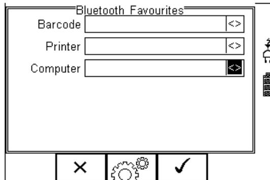
Use the up/down arrow keys to highlight the device type (in this case Computer) then press
