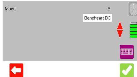
At the end of a test press
