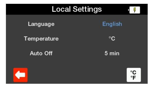
You can then use the up & down arrow keys to highlight the parameter you wish to change and then use the left & right arrow keys to select your preferred setting. There is a fast key on F5 to switch between °C & °F.
