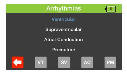
You can then use the left and right arrow keys to highlight the specific arrythmia you wish to simulate. Press down to hilight the amplitude and the left and right arrows to select the setting you wish to use.
