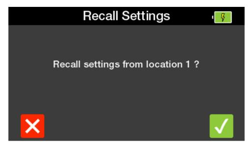
Press the cross on F1 to go back to the settings screen. Press the tick on F5 for yes and the tester will go to the home screen with the relevant settings selected.
