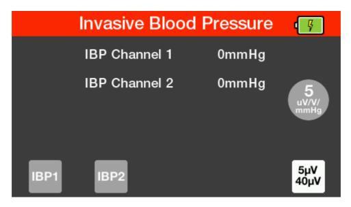
Press F1 or F2 to select the required channel. You can then use the up & down arrow keys to highlight the parameter you wish to change and then use the left & right arrow keys to select your preferred setting.
