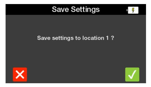
Press the cross on F1 to go back to the settings screen. Press the tick on F5 for yes and the tester will display a message of Saving Settings and then Settings Saved before returning to the home screen.
