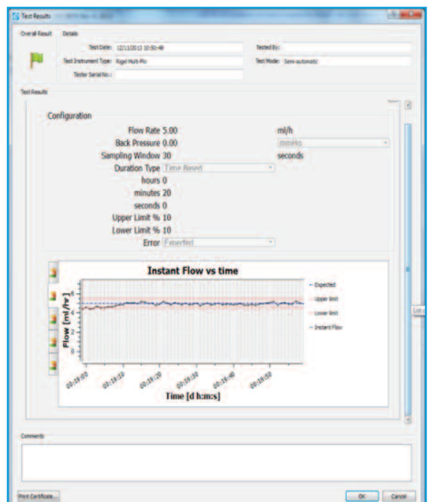
Figure 4: Real-time graphical data in Med-eBase shows whether infusion is within manufacturer’s specification
