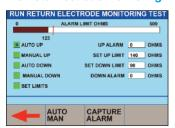
Use the rotary encoder to set high and low alarm points as well as controlling the potentiometer, scaling up or down in manual or automatic mode. Then, simply capture the alarm using the dedicated fast key on the screen. Data will be stored onboard for future traceability.
