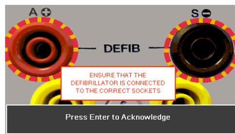
To enter the **Defibrillator Pulse mode** you have to accept the connections warning, using the ↵ (return) key, – the red and black 4mm defibrillator terminals are highlighted with a flashing red / yellow image.
