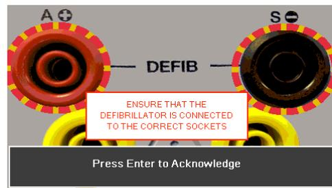
Note 1; to enter the Defibrillator Pulse or AED mode you have to accept the connections warning, using the ↵ (return) key, – the red and black 4mm defibrillator terminals are highlighted with a flashing red / yellow image.
